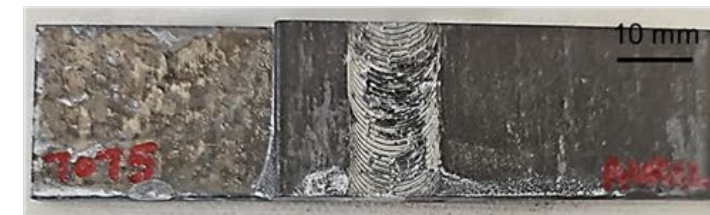
After Corrosion (ASTM B117- 200h) Long term (days-weeks-months) Testing
