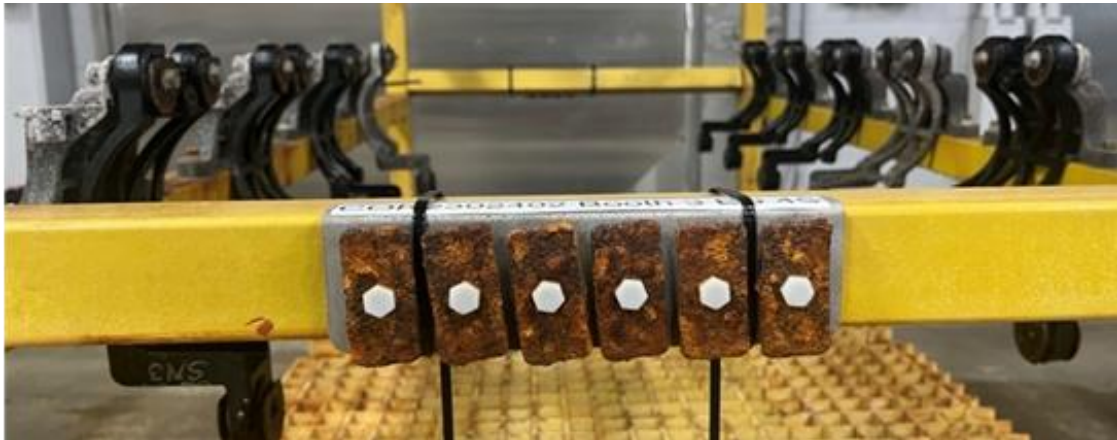
Bare Steel Coupons correlate General Corrosion Mechanism to the Field
