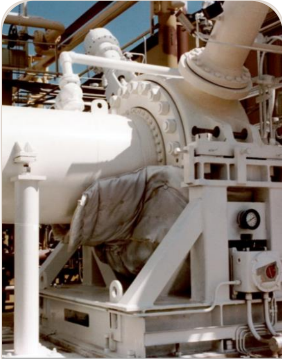
Single-stage Expander EG10 10MW, i-Butane, USA, 1982
