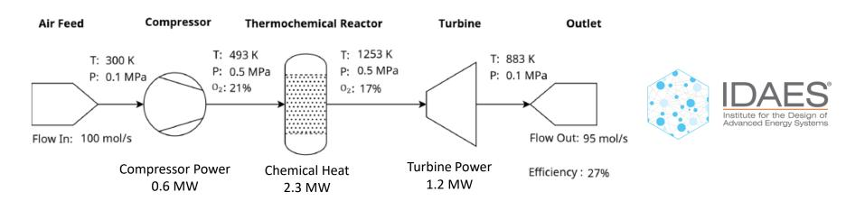
Iron oxide thermochemical storage in simple standalone Brayton cycle.
