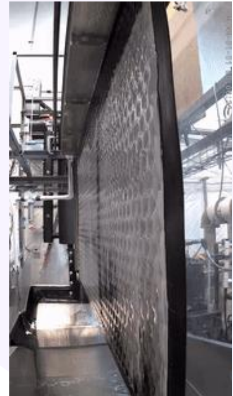
Real-time harvest. Emulsion stops, refrigerant continues to flow, ice pulls away and falls off.
