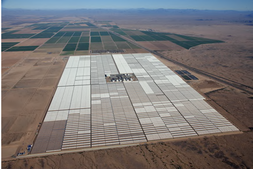
Solana's Generation Station (280 MW e ) 1.5 GWh e Thermal Energy Storage
