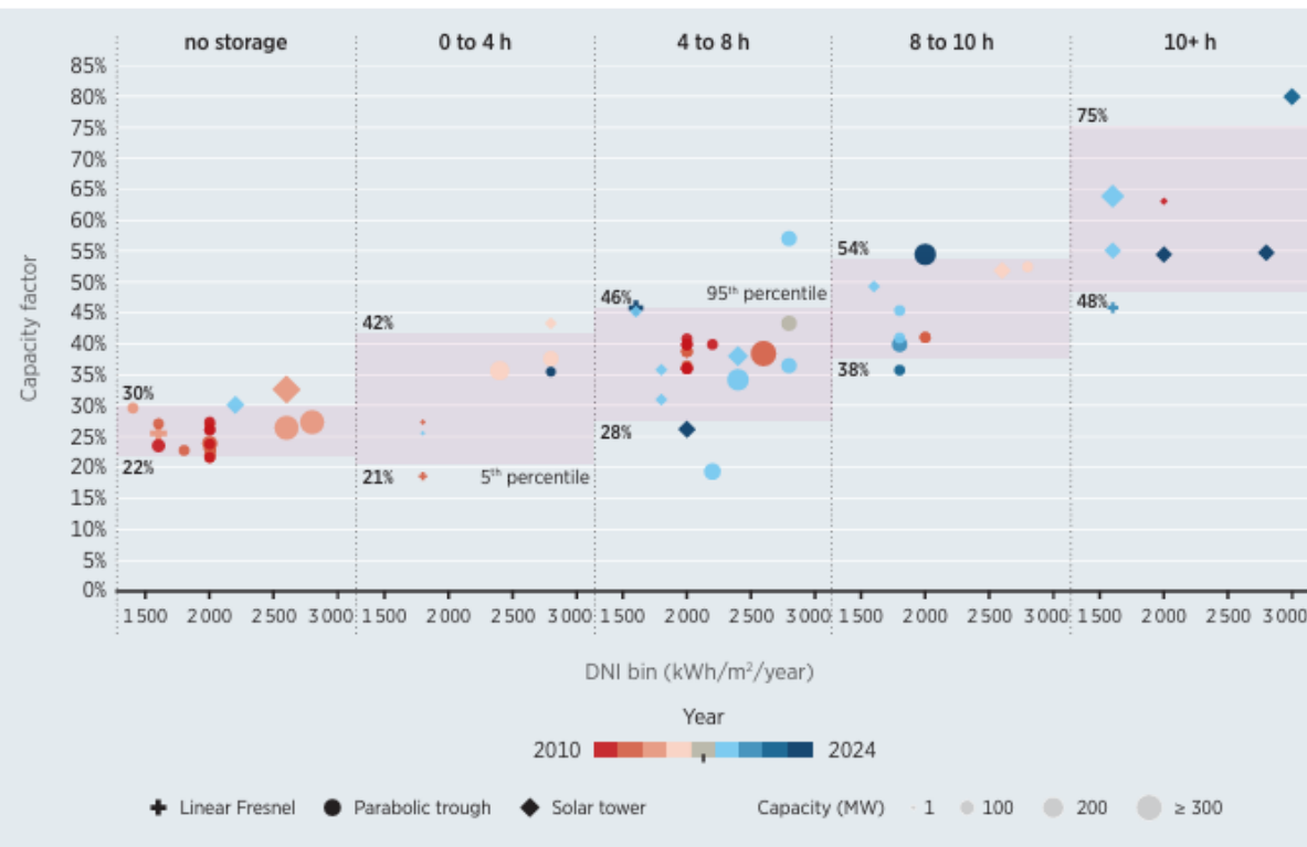
Figure 5.3 Capacity factor trends for CSP plants by DNI and storage duration, 2010–2024
