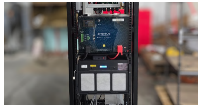
4-9kW Fuel Cell / Supercap System System Design, Integration, and Testing
