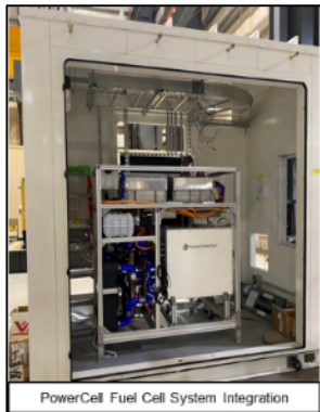
Fuel cell system (left) and inverter (right) integration at GPC
