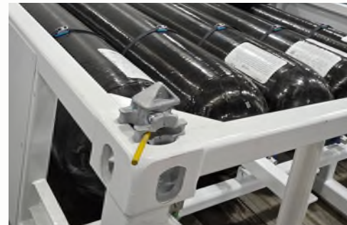
Expandable High pressure storage for cascade filling
