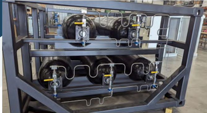
950 Bar Cascade Storage and Refueling System System Design, Integration, Frame Fabrication
