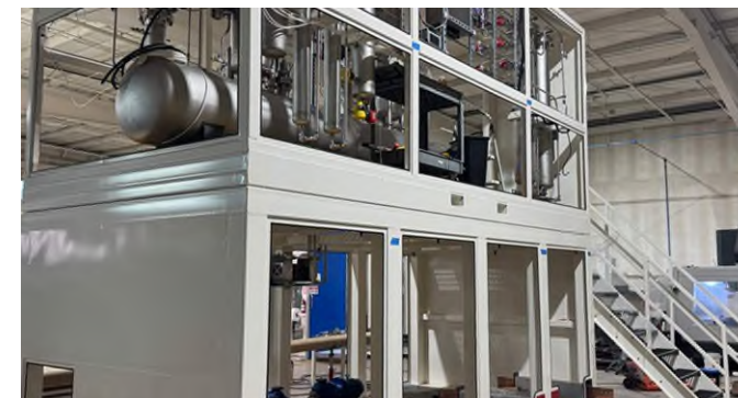
500kg/day Hydrogen Production, Compression and Refueling
